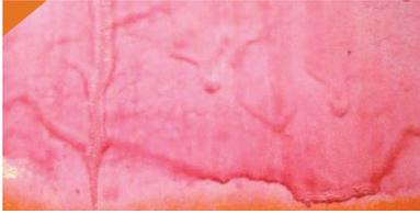
*Sags, runs, and curtains are commonly found on vertical or curved surfaces when the downward movement of paint and coatings pool immediately after application. If the paint or coating is allowed to dry with these defects they result in cracking and peeling.*
