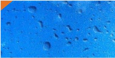
*Outgassing appears as small defects like bubbles, bumps, pinholes, and craters in the coating or paint. Outgassing is difficult to troubleshoot because the defect can appear in a random part of the substrate, or only on a specific spot.*
