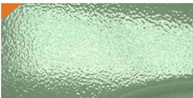
*An orange peel defect is a poor surface texture of the paint or coating that resembles the small, bumpy and rough dimples or pebbled surface of an orange peel.*
