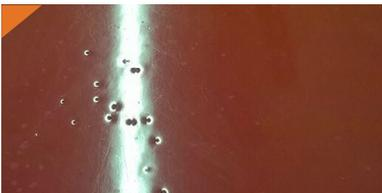
*Pinholes are small cavities, generally less than one millimeter in diameter, that appear over the stopper, filler or other coating.*
