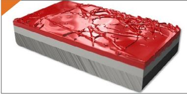
*Cobwebbing, spider-webbing and cotton candy paint defects occur when paint or coating form small droplets that contain too little solvent or thinner resulting in paint particles that leave the spray-tip in a stringy, web-like, filament-like appearance.*
