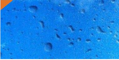
*Outgassing appears as small defects like bubbles, bumps, pinholes, and craters in the coating or paint. Outgassing is difficult to troubleshoot because the defect can appear in a random part of the substrate, or only on a specific spot.*
