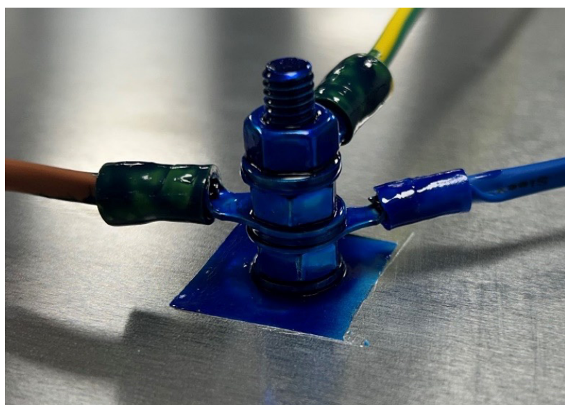
Typical application of Nycote to an aircraft bonding point
